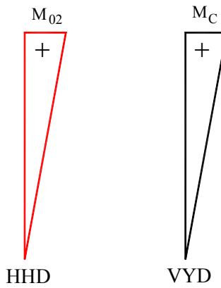
$$w_{12x} = \int_0^{L_C} \frac{M_{02x} \cdot M_{Cx}}{E \cdot J_{Cyx}} dx \quad x \text{ e bağlı momentler:} \\ M_C = \frac{x}{L_C} \cdot L_C = x \\ M_{02} = H_F \cdot L_C = F_E \cdot w_{0max} \\ M_{02x} = H_F \cdot x = \frac{x}{L_C} \cdot F_E \cdot w_{0max} \\ w_{12x} = \int_0^{L_C} \frac{\frac{x}{L_C} \cdot F_E \cdot w_{0max} \cdot x}{E \cdot J_{Cyx}} dx$$
